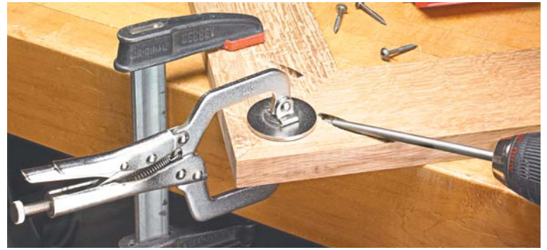
▲ MITER JOINTS Two pocket holes drilled in this small frame secure the miter joint. A face frame clamp makes it easy to hold the joint in position while the screws are inserted.
