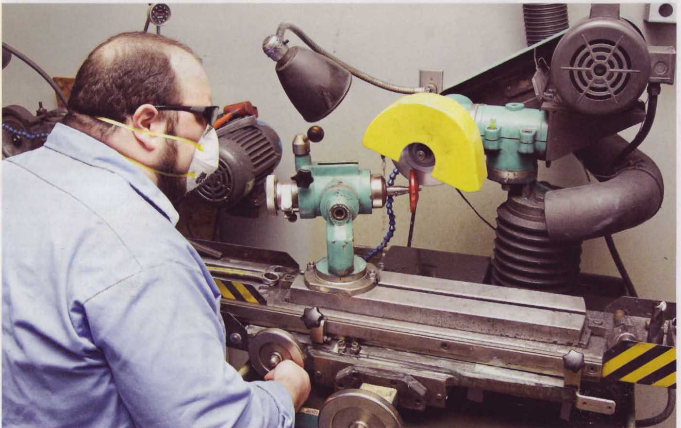
The universal tool grinder shown above is equipped with a divider plate to ensure that both sides of the bit get sharpened equally.
