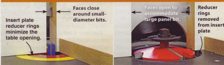
You can adjust sliding fence faces to fully support the workpiece on the infeed and outfeed sides of the cut, no matter what size bit you use. To get the best performance, always set the smallest gap possible around the bit.
