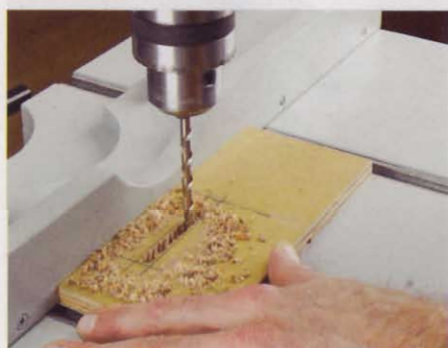
6 Drill out the waste Using a bit \frac{1}{8} " smaller than the slot width, drill overlapping holes inside the layout lines. Drilling an undersized rough slot lets you rout a clean finished-size slot in one easy pass.
