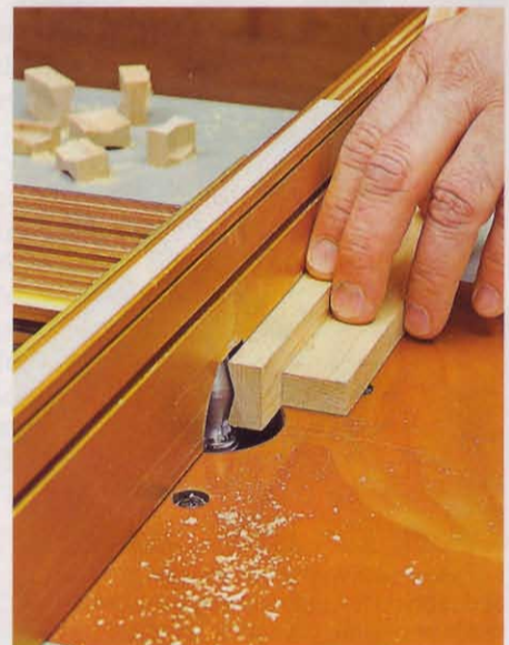
A router makes it easy to embellish your project with decorative effects, such as adding a butterfly spline to mitered joints.
