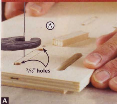
With the slot-end holes drilled, draw tangent lines connecting each pair of holes, and scrollsaw or jigsaw the slots.
