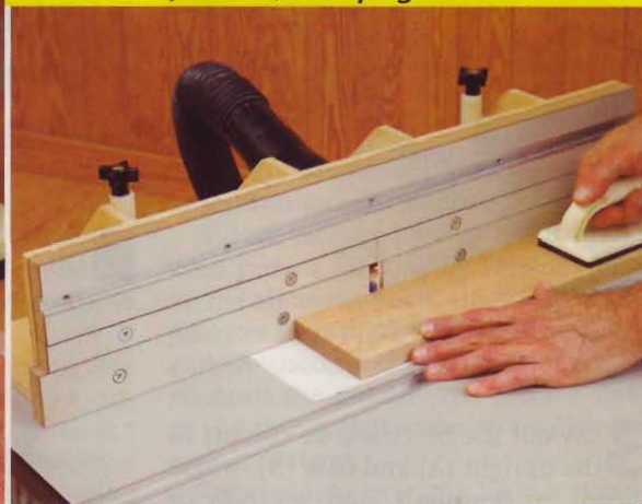
A jointer face quickly straightens edges or removes saw marks for edge-gluing.
