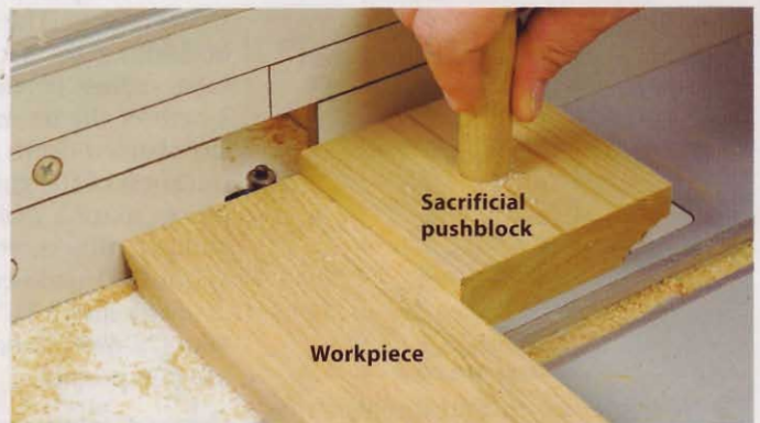
The profile cut into the back edge of this pushblock shows that the pushblock has backed up one router bit already, but still has three more uncut edges left.
