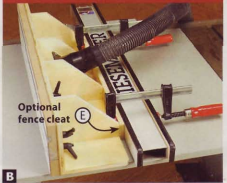
For a tablesaw-extension mounted router, adding the optional cleat (E) allows you to clamp the fence to the tablesaw rip fence.
