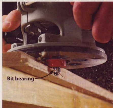
A bearing on this flush-trimming bit rides along the pattern edge and cuts an identical edge on the piece above it. This setup is an excellent way to make finish-quality, duplicate workpieces quickly and without any extra work.
