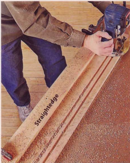
For a low-tech way to cut straight grooves and rabbets in larger boards, use a shop-made or commercial clamp-on straightedge.
