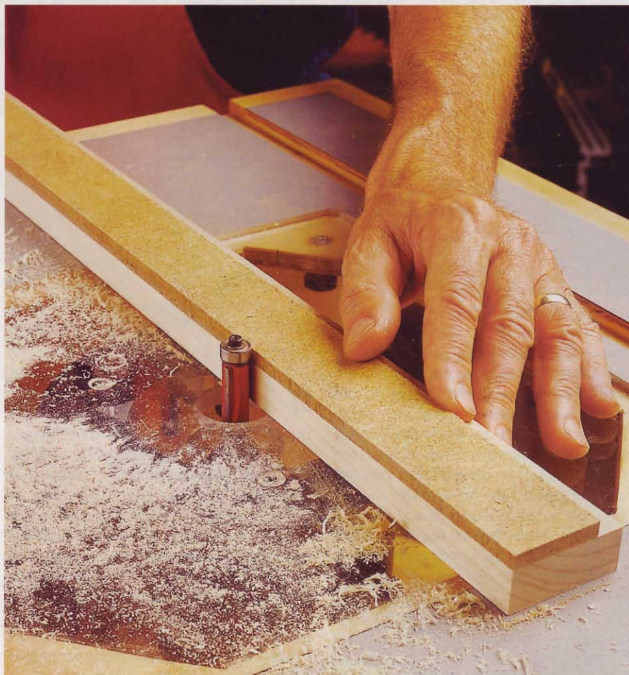
When making identical parts, it's easier to make the cuts faster and more accurate if you use a hardboard or MDF template and a flush-trim bit like the one shown here.
