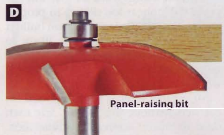
This large-diameter bit cuts the cove profile that "raises" the panel.
