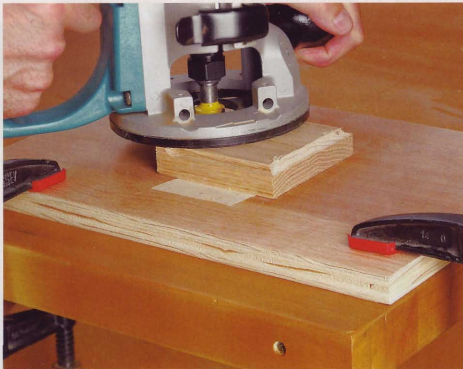
For handheld routing of small parts, clamp a scrap to your workbench, and apply cloth-backed, double-faced tape to the top. Press the part onto the tape for a secure hold during machining.
