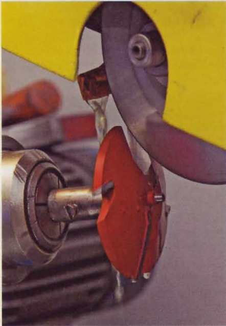
The universal tool grinder shown above is equipped with a divider plate to ensure that both sides of the bit get sharpened equally.
