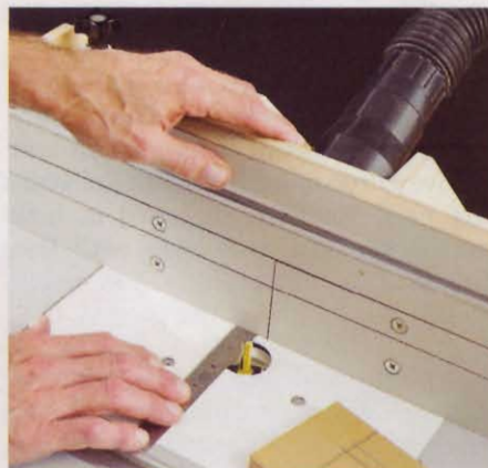
2 Position the fence Chuck a slot-size bit in the router. Place the fence to center the bit in the slot.
