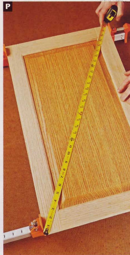
When you cut the rail ends square, and accurately match the coped and stuck profiles, assembly becomes almost automatic.
