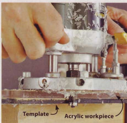
The bearing follows the template to copy the same shape in the acrylic workpiece.
