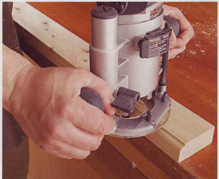
When climb-cutting with a handheld router, limit yourself to bits or cuts that remove only \frac{1}{8} " of material or a slight profile, such as this round-over bit. To remove more material than that, make multiple passes, deepening the cut on each pass.
