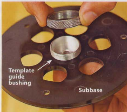
A knurled nut secures the template guide bushing to the bottom of the subbase.
