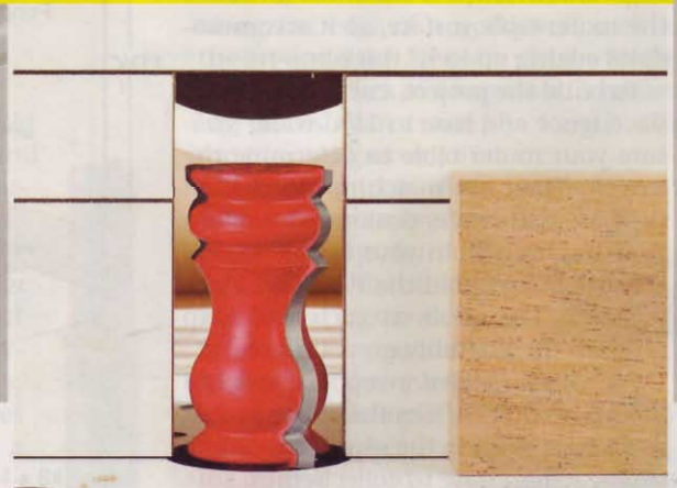
To accommodate tall bits, such as this crown molding cutter, open the 1"-tall center portion.
