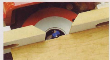
The outfeed side of some fences moves forward with spacers or adjustment screws for edge-jointing boards with a straight bit.
