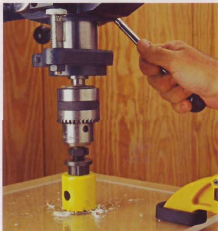
Clamp your insert-plate blank and a backer board to your drill-press table, centered under the bit of your holesaw. Drill slowly, and you'll get a clean cut.
