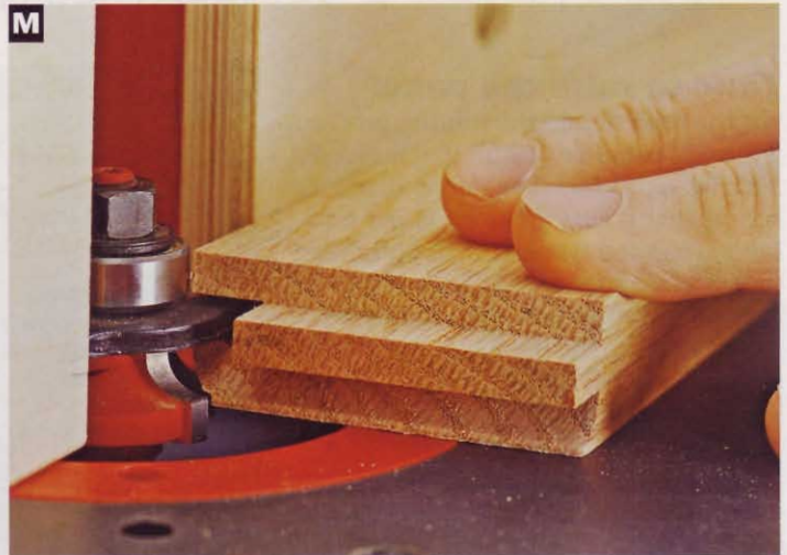
M Make the long-grain cuts on all four frame pieces. Your fingers are close to the bit, so be sure to keep your right hand at the outside corner as you push.
