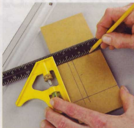
1 Lay out the slot Draw slot boundary lines on the part, extending the end lines to the edges.
