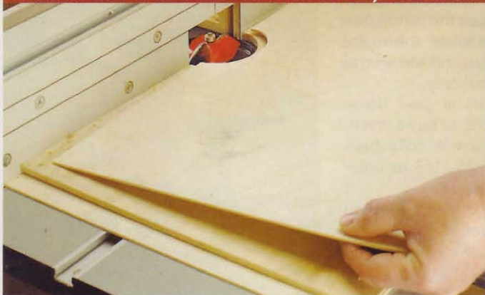
Stack the ¼"-thick spacers on the router table top and secure them with double-faced tape.
