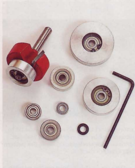
Substituting smaller bearings will allow this rabbeting bit to make wider cuts. The smaller the bearing, the wider the cut.
