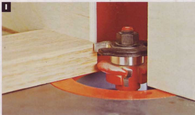
I For the rail-end cuts, set the height of the coping bit by eye. Place the top of its slotting cutter just proud of the workpiece.
