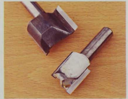
These bits from the WOOD ® magazine workshop showed a lot of wear. Chad used a wire wheel to clean off all the residue before taking them over to the diamond-wheel sharpener.
