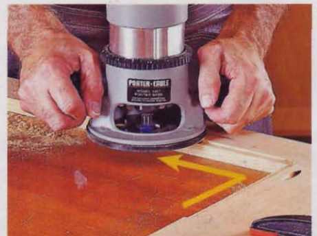
Climb-cutting the rabbet on the back of this frame reduces tear-out.
