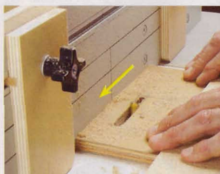
8 Rout the slot Feed the part to the left until it hits the stop. The auxiliary guide keeps the part in line.
