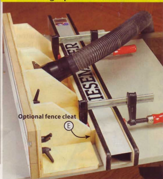
Fence-mounting options include threaded inserts, T-track, and clamps. For a saw-table-mounted router, clamp it to the rip fence.
