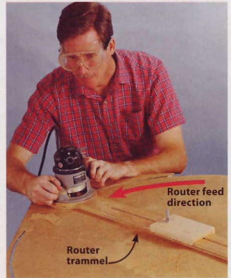
With this circle-jig attachment, you can rout arcs and circles in large workpieces. The trammel becomes a router subbase.
