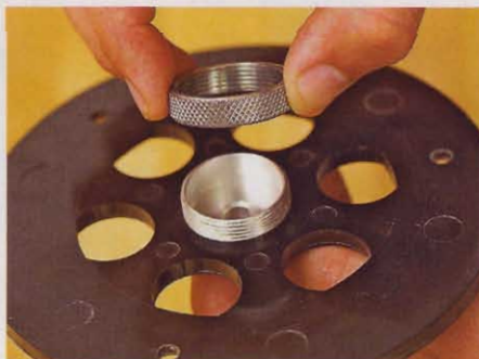
Two-piece guide bushings easily attach to your router base.
