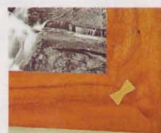
A router makes it easy to embellish your project with decorative effects, such as adding a butterfly spline to mitered joints.
