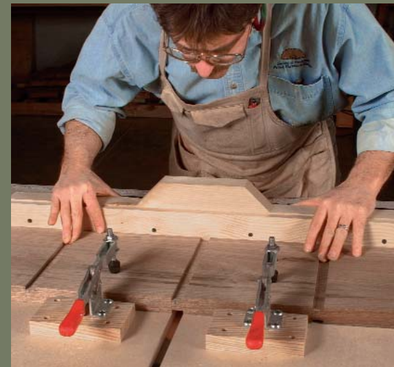
Dado one side at a time. After setting the blades to the right height, make all of the dado cuts on one side of the verticals. Transfer the cut lines for the dadoes on the second side with a square and a sharp pencil.
