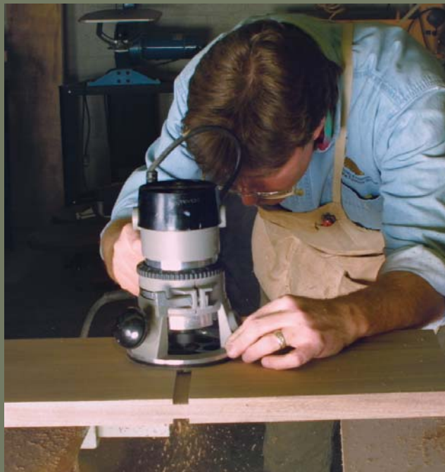
Clean up the sabersaw cut. Use a router equipped with a bearing-guided, flush-trimming bit.
