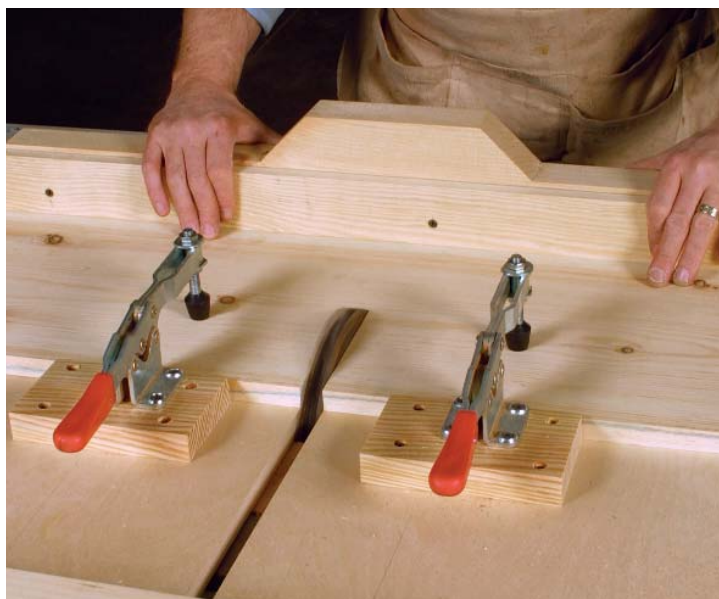
Notch cuts require clamps. While plowing out the notches for all of the shelves, Latta clamps the workpiece in place for each cut, being careful to keep his hands well clear of the exposed dado blades.
