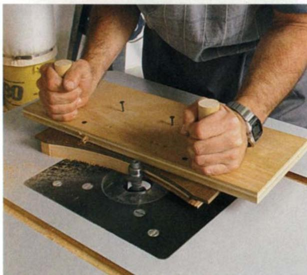
**Cut the profile and curve in one pass.** With the template tacked into place, use a rail-cutting bit to shape the profile and fair the edge.
