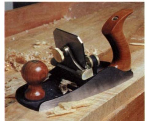
**Big scraping plane from Lie-Nielsen.** The No. 112 scraping plane weighs 4 lbs. and comes with a 2 7/8-in.-wide blade.
