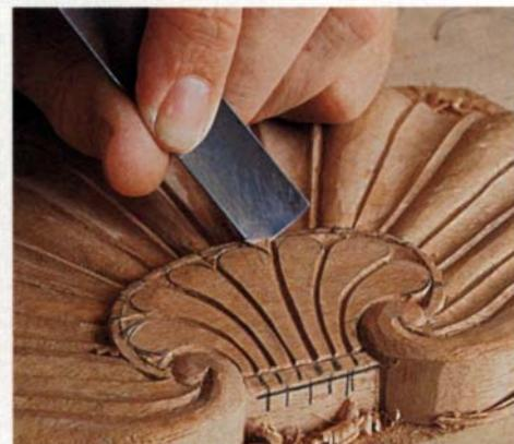
**Chop the tops.** After defining the tops of the petals using a gouge with a tight sweep, the author uses a shallower gouge to remove the triangular chip between petals.
