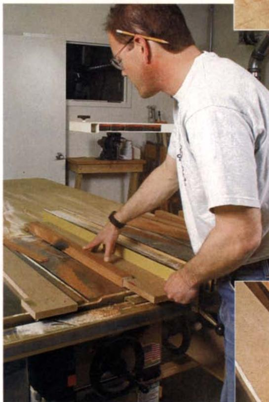
**Color coding can counter confusion. The author marked two perpendicular sides of each billet end with a red pen for the first cuts and a green pen for the second cuts. The jigs are coded the same way. (The first cuts in the billet in the photo have already been sawn away.)**
