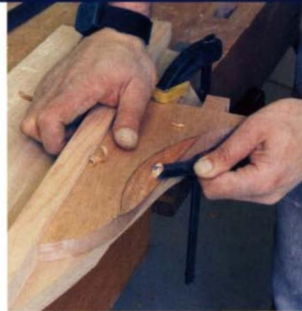
**Fingerhold is cut with a gouge.** The swinging leaf support, cut on the end with a gentle cyma curve, nests against the apron end, which gets cut with a slightly more exaggerated curve. The back of the support is relieved with a gouge to provide a fingerhold for opening the support.
