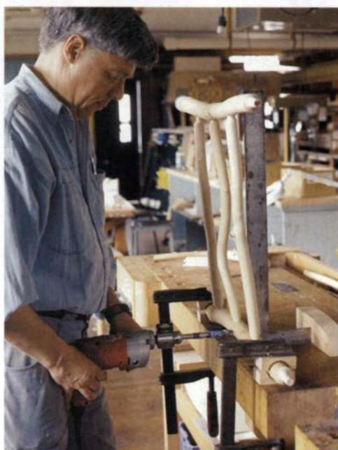
**For angled mortises, tilt the frame, not the drill.** To establish the angle for the side-stretcher mortises, tilt the chair's front frame forward (left). To help measure the tilt, use a framing square held upright in a kerfed block of wood. The author uses shopmade clamping blocks lined with leather to hold the work without marring it.
