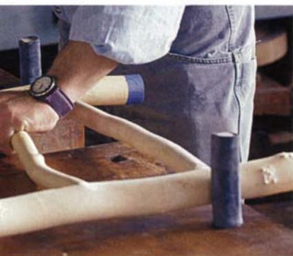
**Putting the squeeze on.** Final assembly begins with the front and rear panels. The author uses a slow-setting epoxy and pulls the joints home with his bench's tail vise and some extralong benchdogs (above). Elbow grease and a rubber mallet are used to drive the tenons of the side rungs and armrests home. Then band clamps hold them in place and a bag of sand across the seat rungs keeps the chair from twisting (right).
