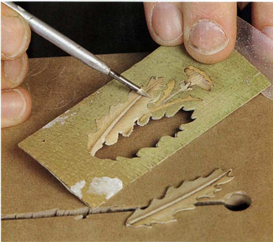
**Leaves fall into place.** Once the first leaf has been completed, place it in the background and secure it with veneer tape. Return to the pattern, align the second leaf and repeat the steps.
