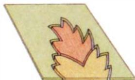
Stack cutting results in a gap between elements the thickness of the sawblade.
