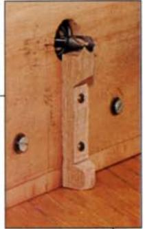
**Cut it "backwards."** Unlike normal routing, these reeds are cut moving the sled right to left so that the bit rotation does not lift the bit and the sled off the table.
