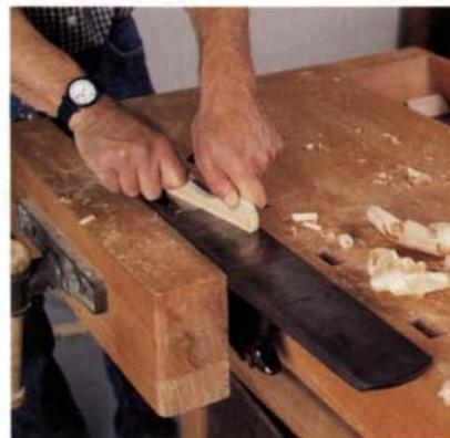
**Jointer plane for straight edges.** The longest of the steel-body planes, a jointer plane, with its 22-in.-long sole, cuts straight edges on long boards (above). Clamped upside down in a vise (left), a jointer plane works well for planing small or odd-shaped pieces of wood.
