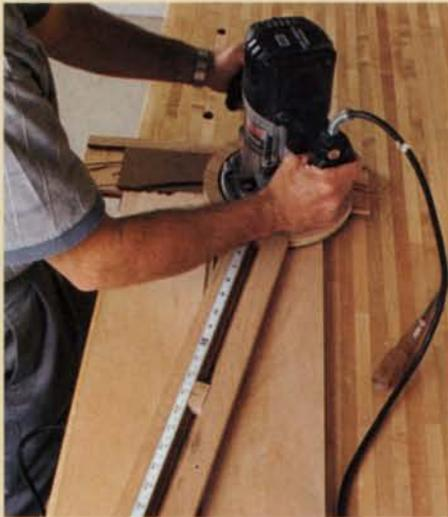
**Making the rail template.** With brads securing the template blank in place, a router outfitted with a  $\frac{1}{4}$ -in. straight bit cuts a smooth arch in the rail template.
