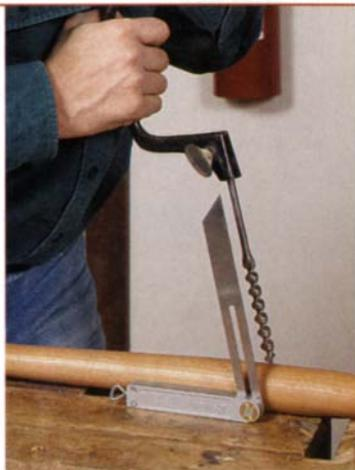
**The auger's lead screw guides the cut.** With its threaded lead screw pulling the bit into the cut, the auger bit requires very little feed pressure. The user can concentrate instead on getting the angle of the hole right.
