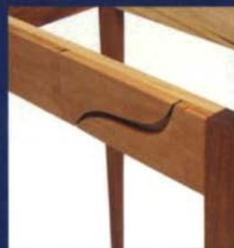
**Metal pin, wood hinge.** The top of the pin is peened to prevent it from slipping out. In operation, the swinging leaf support folds flat against the apron when the table leaves are down.
