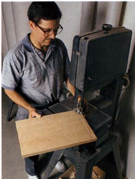
**Cut the panel to rough shape.** Trace the arc from the template onto the panel and trim the waste material away on the bandsaw.
