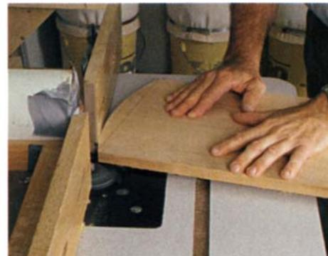
**Raise the panel.** When turning a flat panel into a raised one, you can make a safer cut by using both the fence and the pilot bearing.
