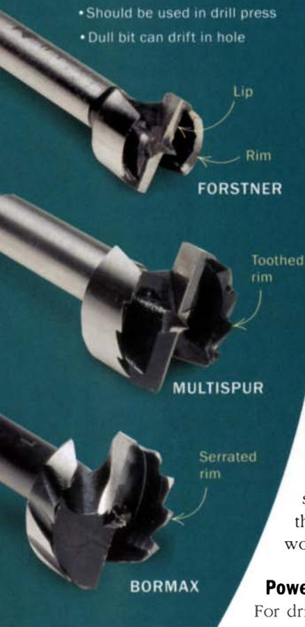
There is a new type of multi-spur on the market, a German-made bit called Bormax. Its teeth are formed by grinding the outside of the rim in a pattern that looks like a serrated knife. This results in teeth with a profile like a typical multi-spur. But the grinding removes metal from the outside of the cutting rim, which is supposed to reduce friction and increase the aggressiveness of the cut.
