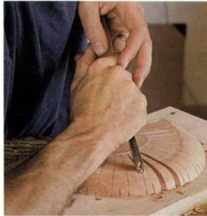
**V-grooves start the fillets.** After redrawing the fillet lines in the ramped area, a parting tool is used to establish each fillet with a V-shaped groove. The groove, centered on the line nearest to the convex lobe, should be about ¼ in. deep at the rosette and deeper as it reaches the perimeter, where it should just erase the shallow bandsaw kerf.
