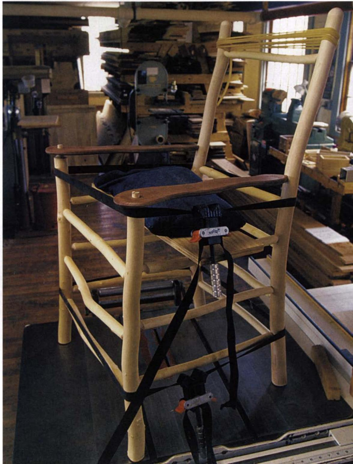
and rear panels (see the photos on the facing page). Brush a slow-setting epoxy in the mortises and use padded clamps to pull each panel together. Padded bar clamps work fine, but I often use my tail vise and some extralong wooden benchdogs covered with bicycle inner tube to avoid denting the chair parts. Once the front and rear panels have been pulled together, I glue in the stretch-
