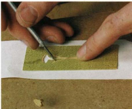
**Using hide glue, tack the stack-cut parts onto white paper.** The gaps left by the blade's kerf will be filled later with dark wax, which creates a sharp, thin outline.
