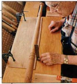
**Next, check and clamp the pattern.** After the bandsawn pattern has been filed smooth, clamp it exactly under the leg. To make shallower reeds at the bottom of the leg, move the end of the pattern slightly toward you.
