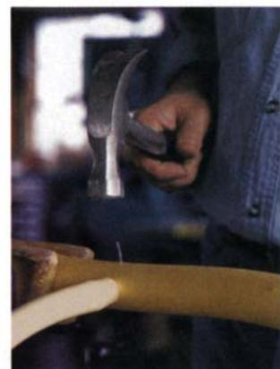
**Mother Nature's tenon pins.** Thorns harvested from the hawthorn tree are excellent for pinning tenons. No machining is needed; just drill and drive.
