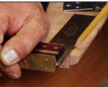
**Hinge pivots at the roundover fillet line.** Transcribe a line on the underside of the tabletop equal to the setback of the vertical fillet on the rule joint.
