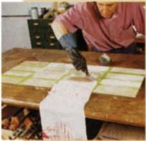
I put four different kinds of chemical strippers to the test on an old, painted piano bench. Using the tissue test, I found the top finish to be lacquer, but the tests for the paint underneath were inconclusive, so I assumed it to be an oil-based paint.
