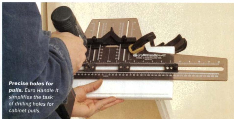
**Precise holes for pulls.** Euro Handle It simplifies the task of drilling holes for cabinet pulls.
