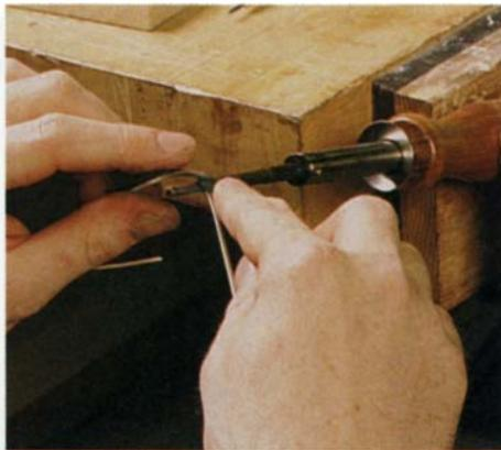
**Bend the stringing using a soldering iron set on low.** A feeler gauge helps nudge the stringing into shape. The author modified his soldering iron's tip by adding different-diameter brass tubes slid inside each other.
