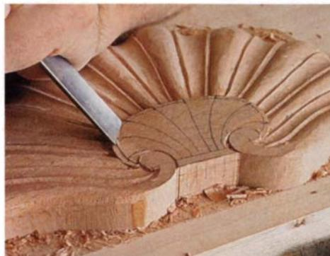
**Shape and shave the rosette field.** Using a gouge with a shallow sweep, the author defines the narrow, curving rib at the rim of the rosette. Then, after he chops in the volutes, he uses a wide chisel to angle the whole field of the rosette, ramping it downward from the rim toward a line between the volutes drawn  $\frac{3}{16}$  in. below the high point.
