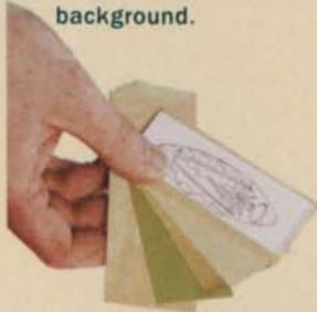
**Veneer sandwich.** Holly, satinwood and green-dyed holly are placed between two-ply veneer to prevent tearout.
