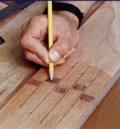
**The drop-leaf supports swing on a wood hinge.** Hinge knuckles—two on the support and three on the stationary piece—are  $\frac{5}{8}$  in. long. The width of each knuckle is determined by the width of the apron stock divided into five parts. A cyma curve on the end of each support adds a decorative touch.
