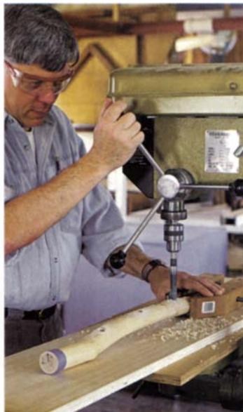
**Flat clamp tames a wild workpiece.** To make a curved chair leg fit for safe, accurate mortising on the drill press, attach a hand-screw clamp to one end. The clamp holds the leg in register and provides a flat surface to mate with the table. To get mortises of the same depth, use the index on the collar of the drill-press arm.
