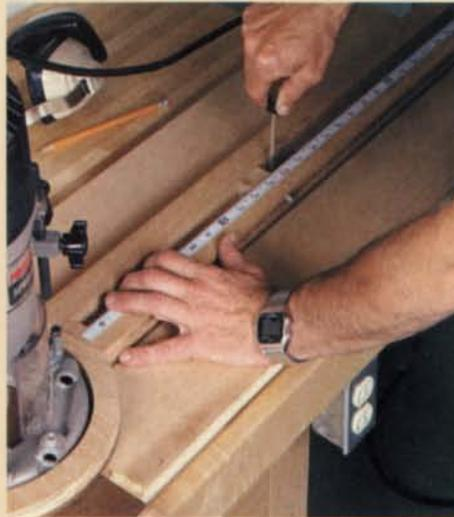
**A slight adjustment.** To cut the panel template, increase the radius on the jig's arm  $\frac{1}{2}$  in. to allow for the bit diameter and the panel tongue.
