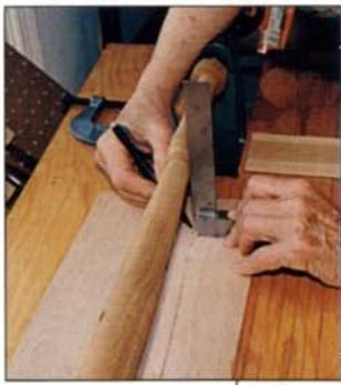
**First, drop a line, but make sure it is true.** Using a square, drop a perpendicular repeatedly from the turning to the pattern blank. Connect the points and bandsaw carefully so that the pattern profile is the same as the turned leg.
