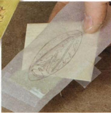
**Make a tracing and flip it over.** Slip a leaf assembly into position. Using carbon paper, transfer the pattern of the leaves onto the veneer.
