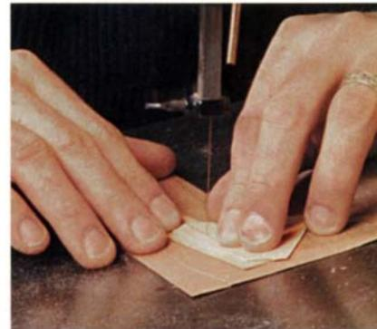
**Using clear tape, attach a vein to one half of a leaf. Tilt the scroll saw's table to about 13°. Cut the first half of the leaf's vein. Bevel cutting will produce a very snug joint between parts.**
