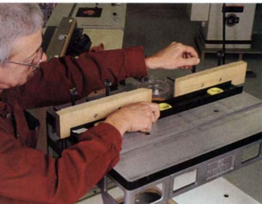
**A fence should be square to the table and easy to adjust. A split fence, which is found on many benchtop models, such as the Woodstock Rebel, must be realigned each time it is moved, a time-consuming process.**
