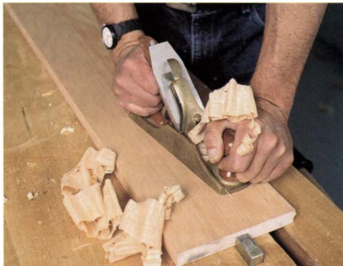
**After the jack, use the smooth.** A smooth plane is used for the final dressing of the face of a board. The plane is especially handy for removing the marks left by jointers and thickness planers.
