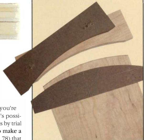
cabinet doors. An arch of less than 1 in. leaves the rail too meaty and the arch too subtle. Making an arch with a depth of more than 1 in. cuts down on rail width so much that it appears weakened.
