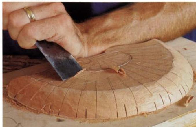
**A gentle ramp.** After defining the perimeter of the rosette at the center of the shell with  $\frac{1}{8}$ -in.-deep chops with a gouge, the author wields a straight chisel bevel side down to create a ramp, a slight rise from the rosette toward the perimeter.
