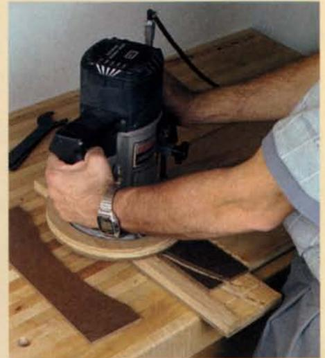
**A matching pair.** Once the radius has been adjusted, tack a Masonite blank onto the jig's well. Cut the panel template with the router in a single pass.
