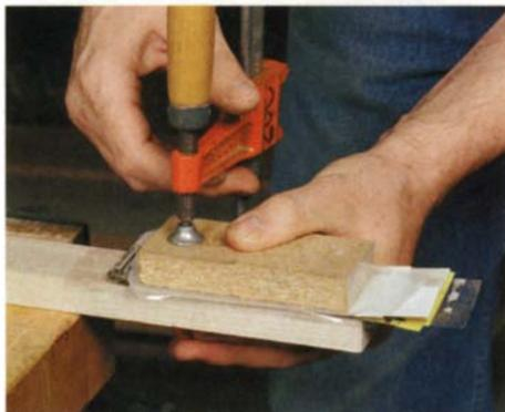
**Gluing and clamping.** After gluing a piece of onion-skin or tracing paper to the face of the partially completed oval, clamp it between blocks of wood. Veneers come in many thicknesses. To even out the pressure when clamping mixed stock, use strips of newspaper.
