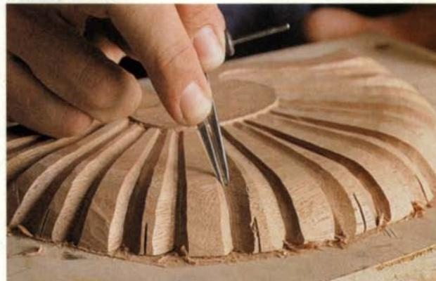
**Finishing the fillet.** With dividers or a compass set at ⅜ in., the author scribes the width of the fillet from backer board to rosette (left). One leg of the dividers rides in the bottom of the V-groove, the other on the concave-lobe side of the V-groove. With the parting tool, he makes a shallow cut to the concave-lobe side of the line (below left). This cut both defines the fillet and starts the wall of the concave lobe.
