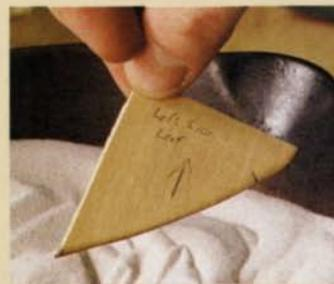
**Mound, then dip.** Mold the sand into the shape of the piece. Dip the part for a few seconds at a time, checking it frequently.
