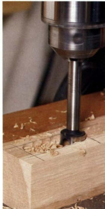
**All-terrain bits.** Steep angles, overlapping holes, very thin stock—none of these situations poses a problem for the Forstner bit, with its continuous rim guiding the bit. Unless the bit is backed out of deep holes every ⅛ in. or so, chips become impacted above it and can cause burning.
