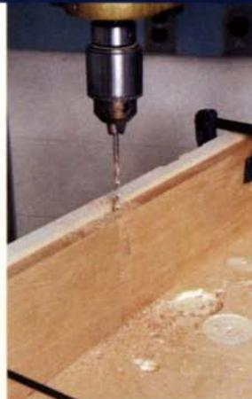
**Fit to be drilled.** Once the wood hinges have been pared to fit, clamp the pieces together against a backer board and drill a  $\frac{1}{8}$ -in.-dia. hole through the hinge. A  $\frac{1}{8}$ -in.-dia. steel rod is used as a hinge pin.
