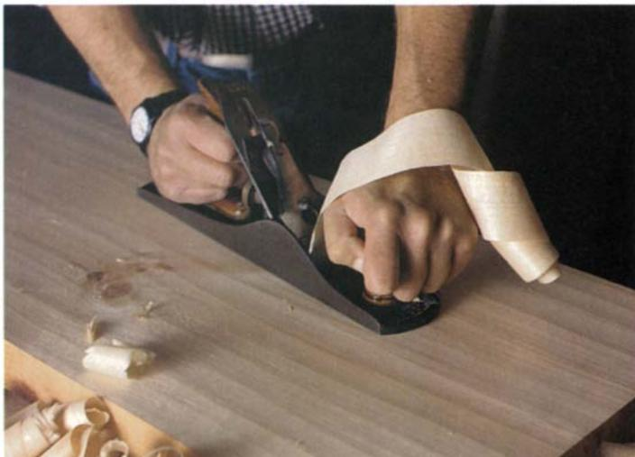
**Face-planing starts with a jack plane.** A jack plane, sharpened with a slight crest in the iron, makes quick work of dressing a roughsawn board. The telltale scalloped surface is a sure indication of handwork.
