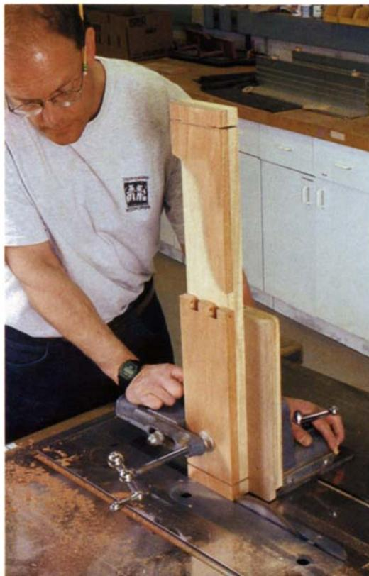
**Table aprons are double thick.** After the swinging leaf support has been cut, fit and drilled and the end of the apron is cut with a cyma curve, the primary apron pieces are glued to subaprons. Cutting tenons on the doubled-up aprons is straightforward. In the photo, the swinging support has been removed from the apron.
