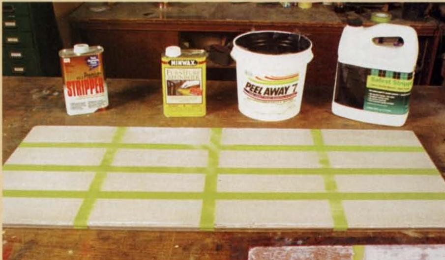
**Before and after.** The author tested four categories and brands of commonly available strippers. He checked and compared the results after 30 minutes, one hour, three hours and six hours.
