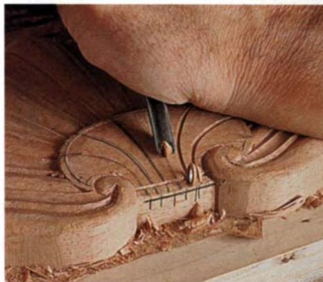
**V-grooves stop at the bar.** Parting-tool cuts define the petals of the rosette, starting at the rim and ending at a  $\frac{1}{8}$ -in.-wide bar at the base of the ramp.
