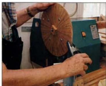
**Reeding a turned, tapered, Sheraton-style leg starts with a wheel.** After the author turns his leg blanks, he leaves them on the lathe. A plywood wheel attached to the lathe's outboard faceplate keeps track of the stops every 30° for each of the 12 reeds.
