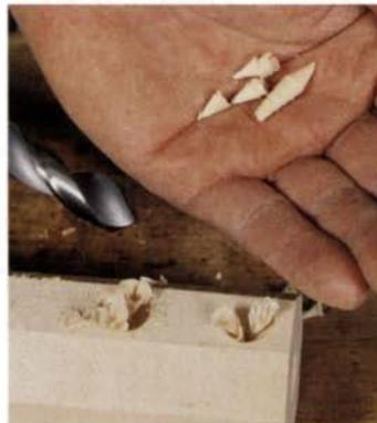
**Long-point twist drill takes a sweet shaving.** Ground to a 90° V-angle at the tip and sharpened properly, a twist-drill bit should cut cone-shaped shavings.
