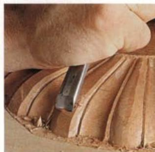
**The ins and outs of lobes.** Grain orientation on all but the center lobes will usually necessitate cutting toward the rosette on one side of the lobe and away from it on the other.
