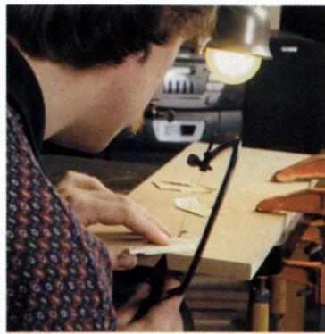
**Cut carefully.** Keep the fretsaw blade angled at about 13° and cut slowly and steadily, turning the stock as needed. Note the plywood support with a bird's-mouth cutout.
