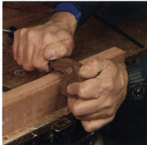
Filing a cutter to shape —Almost any profile, up to 1 in. wide, can be filed into blade blanks made from old cabinet scrapers, sawblades or new blank stock (above).
