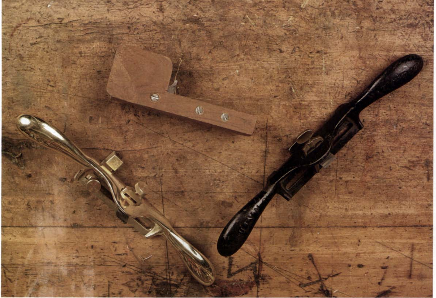
Scratch stocks—old, new and shopmade—Whether old like the Stanley #66 (right), new like the Lie-Nielsen #66 reproduction (left) or shopmade (top), these scratch stocks are a simple way to reproduce moldings or create new designs accurately and economically.
