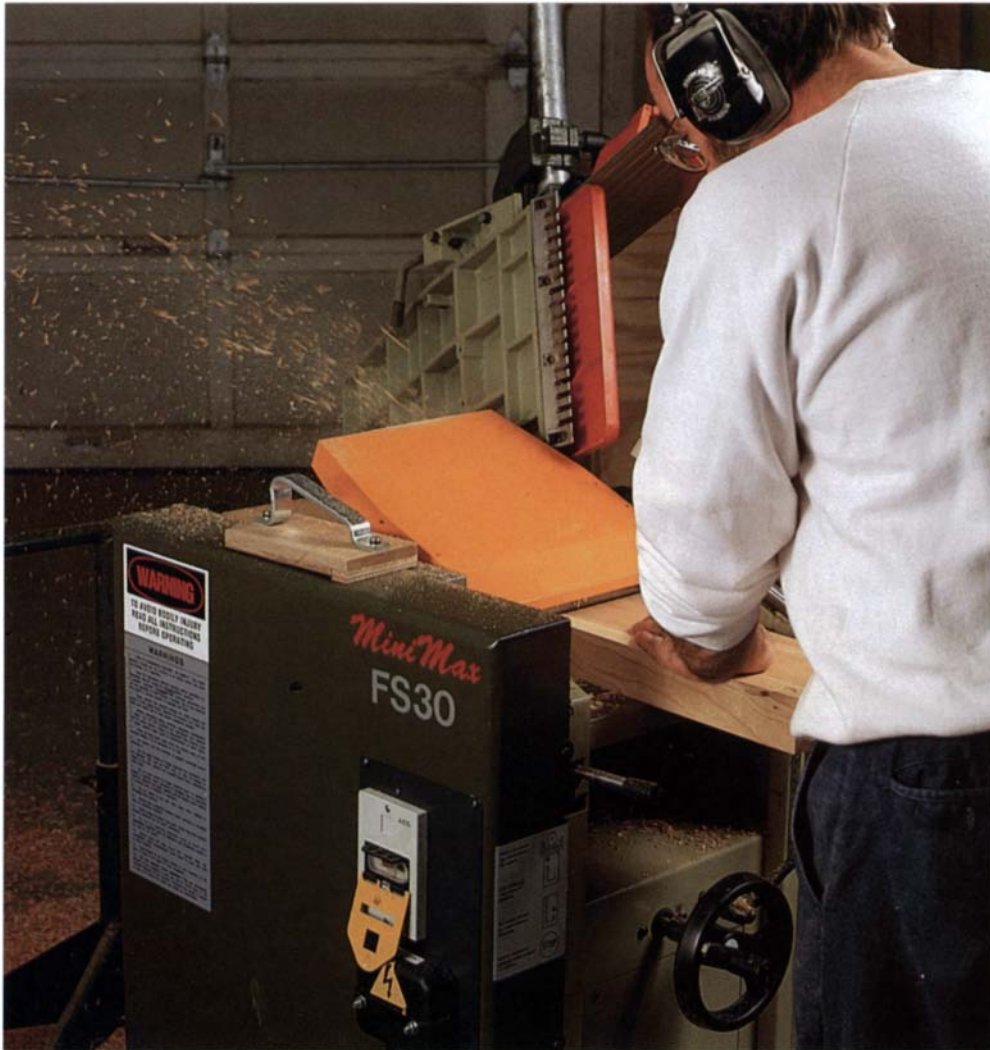
The MiniMax can plane and face-joint boards nearly 12 in. wide. With the MiniMax FS 30's jointer tables up, FWW publisher Jim Chiavelli thickens a piece of 16/4 cherry.
