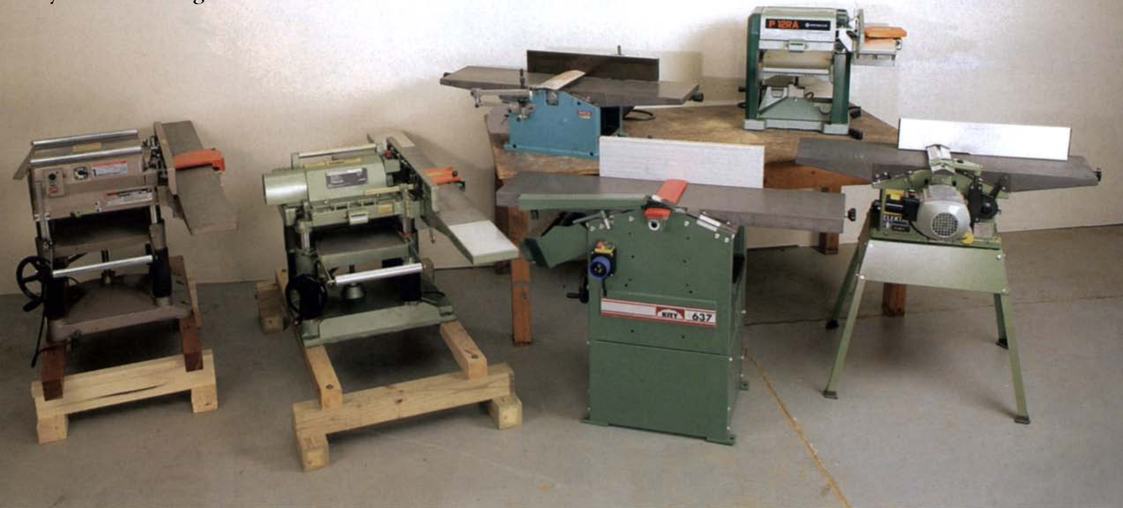
Two types of jointer-planers: Side-by-side models include Makita's 2030N and Hitachi's F-1000A and P 12RA (1st, 2nd, 5th from left); over-and-under units are Inca's 570, Kity's 637 and Elektra Beckum's HC 260-ESH (3rd, 4th, 6th). Two others are below and on the facing page.
