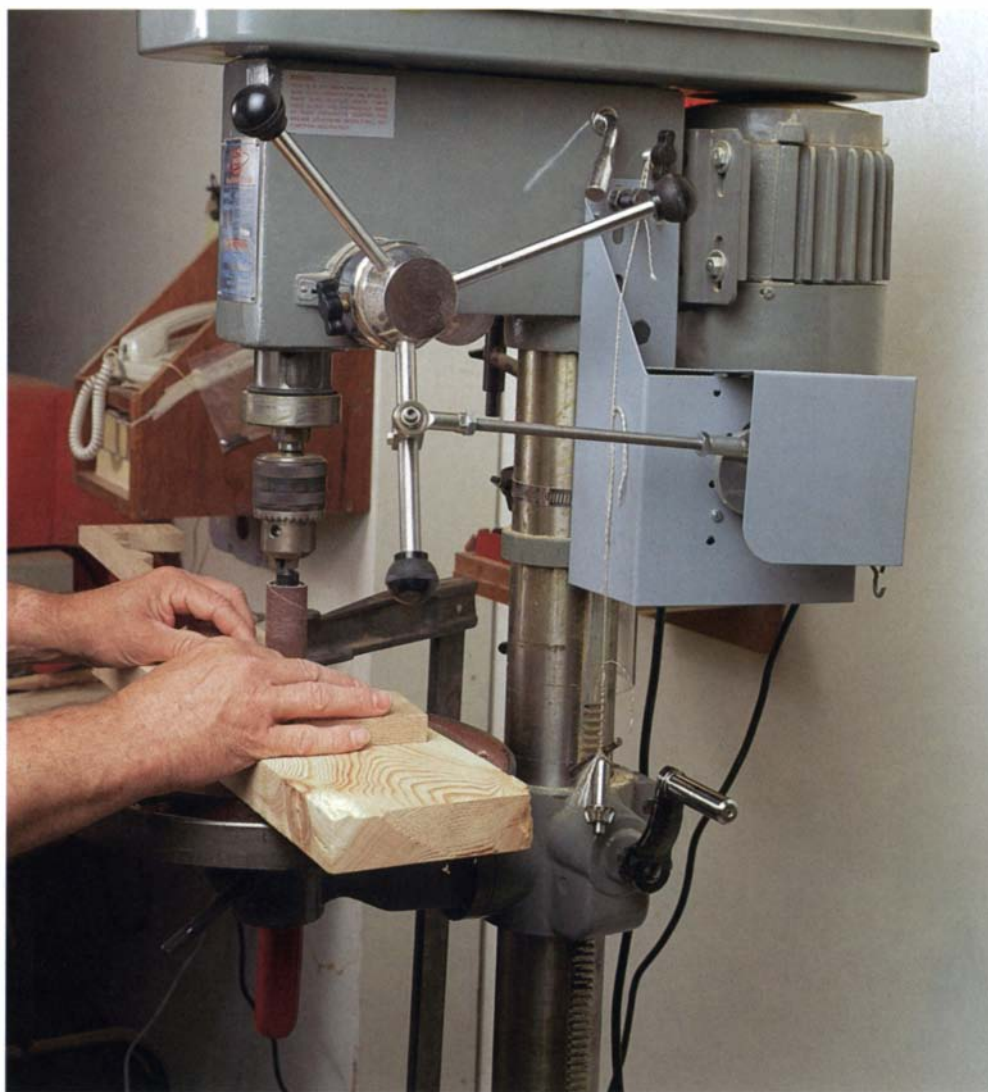
Big benefit in a compact package. GP-Designs' oscillating spindle-sander attachment connects to almost any drill press and provides oscillating spindle-sander function without compromising the drill press's main function: drilling. The retrofit unit sells for $169.
