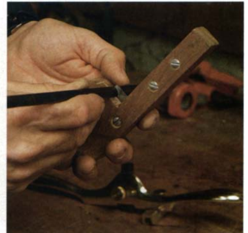
Matching a molding to a cutter (below) is crucial to reproducing old moldings. File the cutter to the negative image of the molding. Check the cutter frequently while filing to make sure it is an accurate match.
