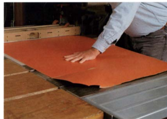
Simple extrusion guides laminates securely through tablesaw blade. The aluminum guide keeps sheets of laminate from slipping under the rip fence or riding up on the blade as the laminate is ripped.
