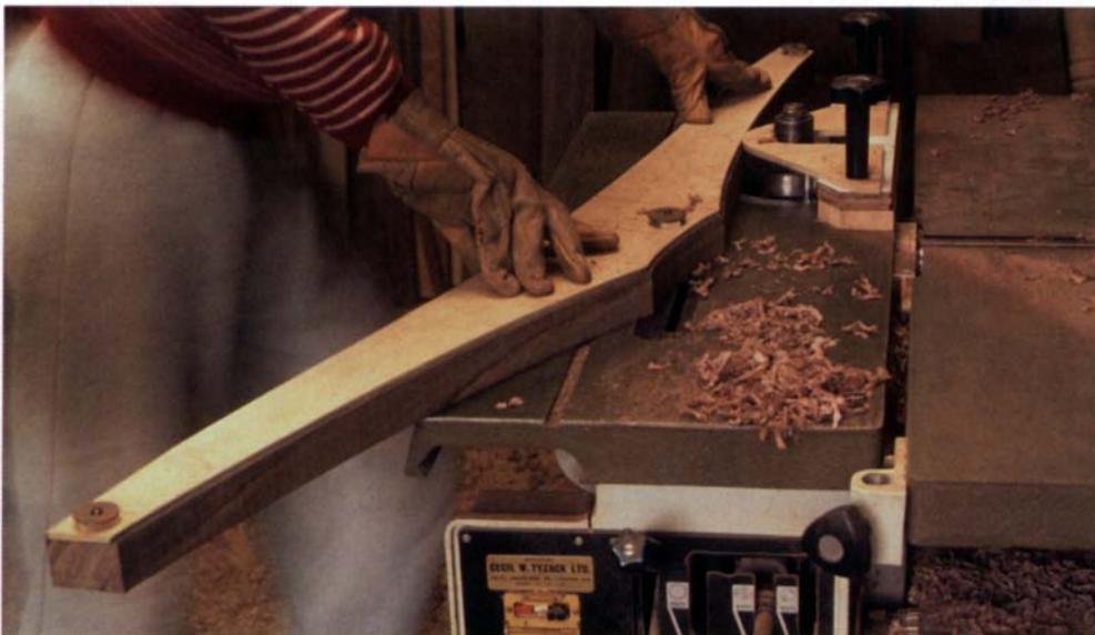
Ring fence makes shaping easier —It's easier to spindle-shape curved pieces with a shop-made ring fence that follows a template attached to the stock.
