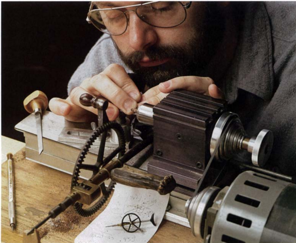
Wee machines make wee tools —Using his precision mini-lathe (left), William Robertson shapes a match-head-size knob for a miniature hand drill (foreground). The full-scale original is placed so he can copy the handle profile.
