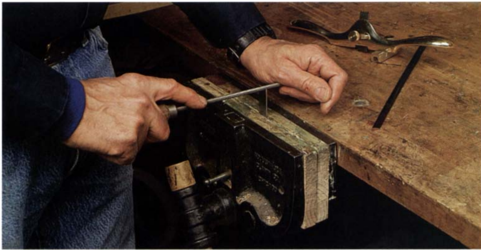
Filing a cutter to shape —Almost any profile, up to 1 in. wide, can be filed into blade blanks made from old cabinet scrapers, sawblades or new blank stock (above).
