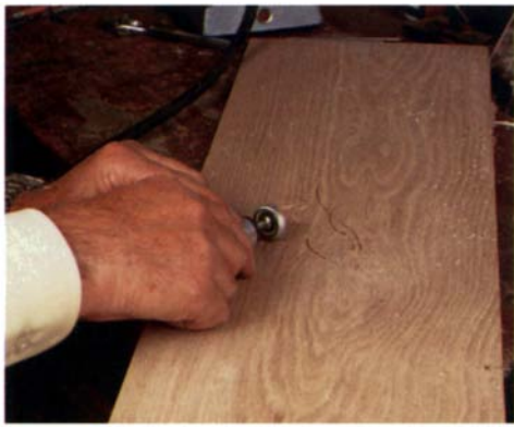
Adding details —A key-seat cutter ground to 45° carves the leaves and petals. Handle the cutter carefully, and be sure it has stopped before you put it down.
