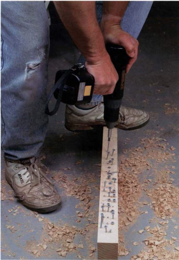
Every one of the drills was able to bury 3-in. drywall screws into hard maple, as long as a screw didn't snap or become stripped. Many did. Drills were run in the low-speed (high-torque) range.
