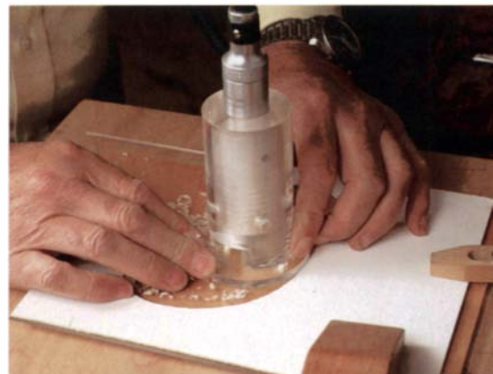
Routing acrylic templates—The author holds the router firmly against the poster-board guide to rout an acrylic template. A separate template is needed for each flower stem or branch in the design.
