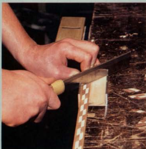
A small miter box and a Japanese backsaw work well for cutting miters at corners and for splicing the banding. A Western-style backsaw also works just fine.
