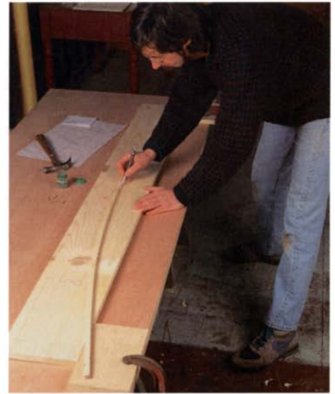
Bending a batten to points along a curve is the best way to lay out long, gentle curves. For fair curves, use a square batten.
