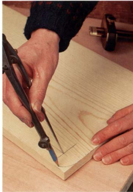
Laying out round corners is easy with marking gauge and compass. Set both for the same radius, mark intersecting lines with the gauge, and you have a pivot point.
