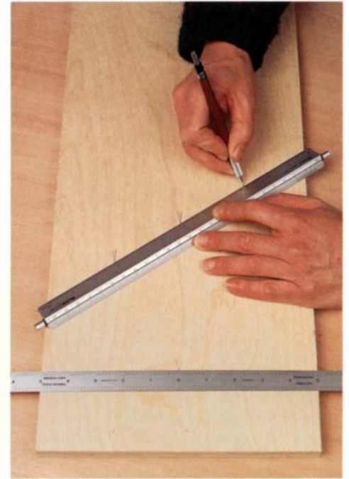
Centering rules and regular rules are both useful for locating centers. They can also be used for establishing regular intervals across a board's width.
