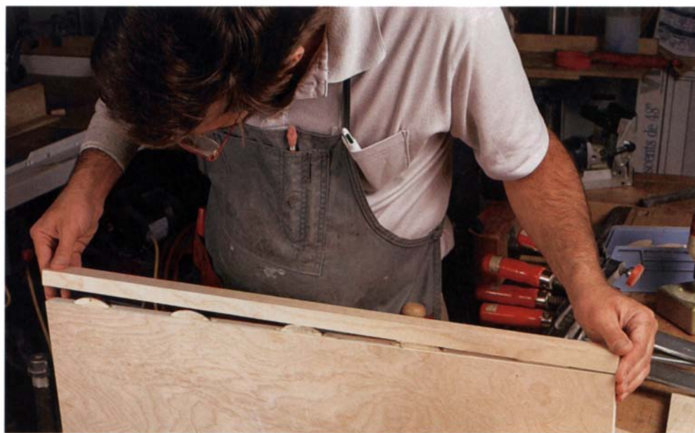
A plate-joined strip of hardwood trims the CPU cabinet side (above). The biscuits strengthen the joint and keep the pieces aligned during assembly.
