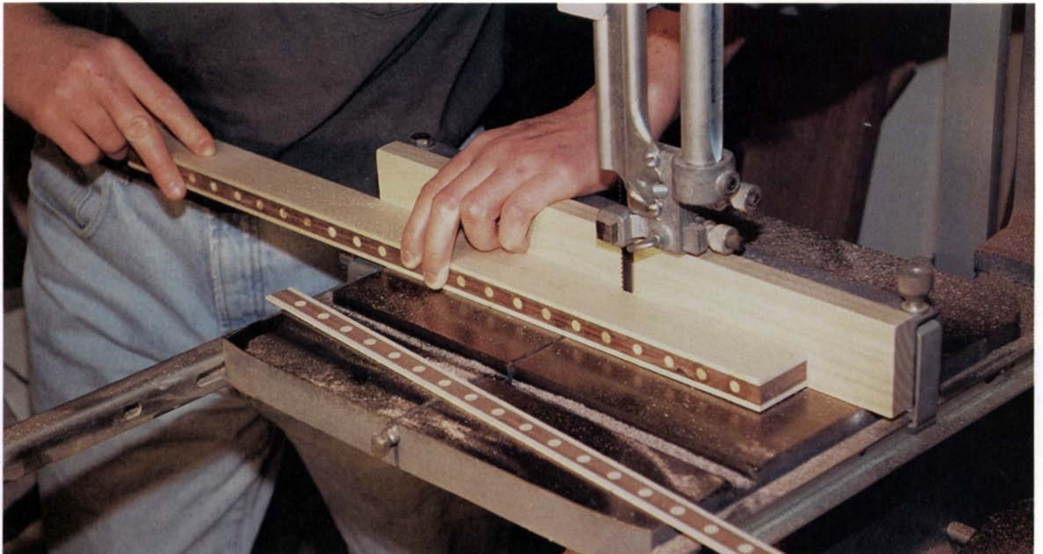
Inlay bandings are sliced from a board that has been made for that purpose. Cutting bandings on the bandsaw results in less waste than cutting them on the tablesaw. It's also much safer on the bandsaw because there's no danger of kickback or of the blade binding.
