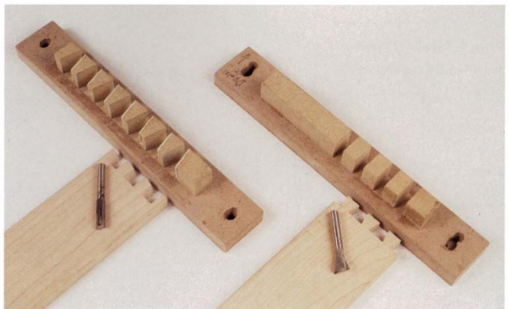
Matching templates and bits— As a sample of his jig's versatility, the author displays mated templates and corresponding bits. For adjustment, the mortise-and-tenon pattern (left) has a screw-on tenon and a mortise-shortening insert. The pin-and-dovetail templates produced the joinery examples above. When indexed by the tail pattern, the jig can also cut finger joints; simply swap a straight router bit for the dovetail bit.
