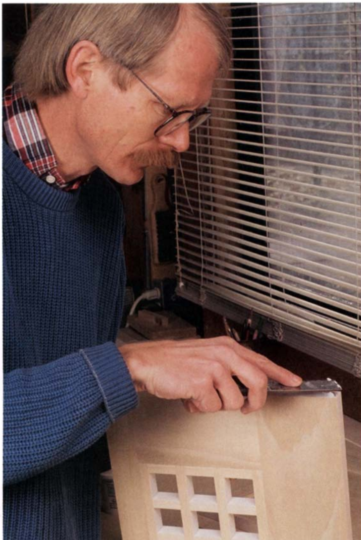
Even with end grain, it's best to scrape off most of the spackle. If necessary, apply a second time rather than build up a thick layer. Do a last round of filling when the piece has been primed. The layer of finish will highlight any imperfections.
