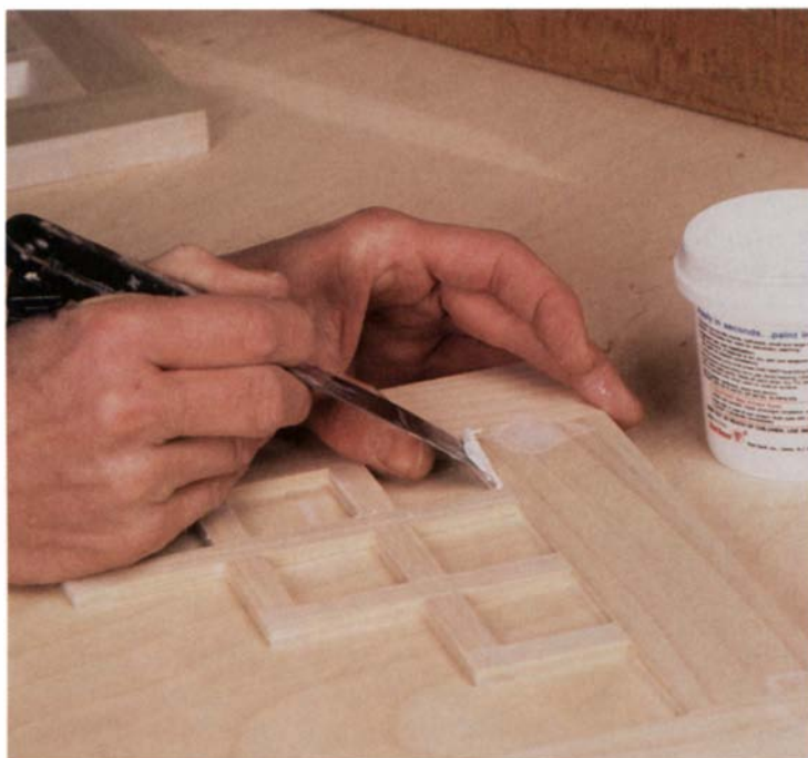
Fill every corner, whether you can see a seam or not. For long runs, caulk is best, but in tight quarters, like the door panel grids, the author uses spackle because it's less messy. With a freshly filed putty knife, he removes 95% of the filler he lays down.
