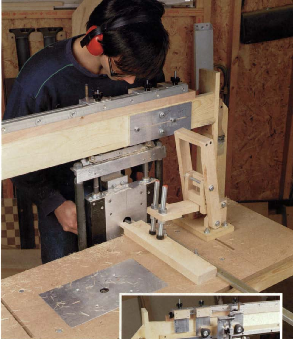
Guy Perez routs a tenon using a shop-built jig. Unlike jigs that require an operator to move control levers and machine, Perez's jig fixes the work, which lets him rout with two hands. The back of the jig (inset) reveals a carriage that guides both vertical travel (rods through bushings) and horizontal motion (rails captured by bearings). The router's plunge mechanism sets depth of cut.
