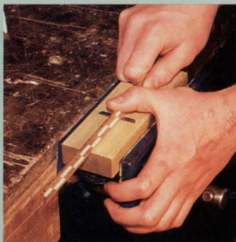
An inverted block plane with a very sharp blade is just the thing for shaving off tiny curls to get a piece of oversized banding to fit.
