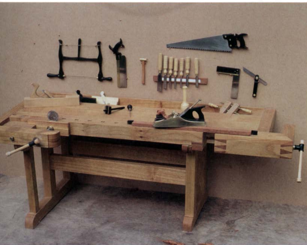
Magnum opus in teeny tools —From the sliding bevel on the right to the shoulder vise on the left, all the tools in this photo are functional as well as fractional. About one-quarter scale, most are made of ebony and boxwood. The Norris plane infill is rosewood and is a working model; the shavings shown in the photo were actually made with it. The plane was made from a set of engineering drawings from a replica kit produced by R.H. Wood.
