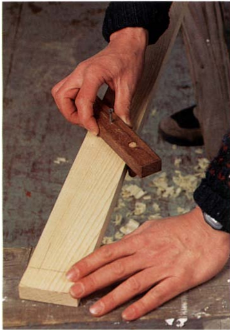
An effective and cheap centering scribe can be made from a piece of scrap wood, two dowels and a drywall screw, as the author demonstrates above.
