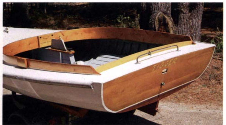
Decent bending characteristics convinced the author to use elm to frame his sailboat. Discovering that early boatbuilders used elm nearly as much as oak, Textor replaced the vessel's ribs and her transom with elm. Paint and marine varnish help protect the wood against the elements.
