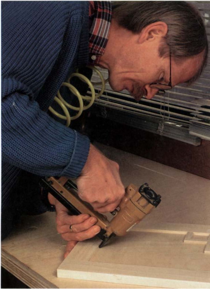
Nail in the rail —The author shoots brads through the frame of the door to keep it from shrinking away from the panel, which could crack the paint and expose unfinished wood.
