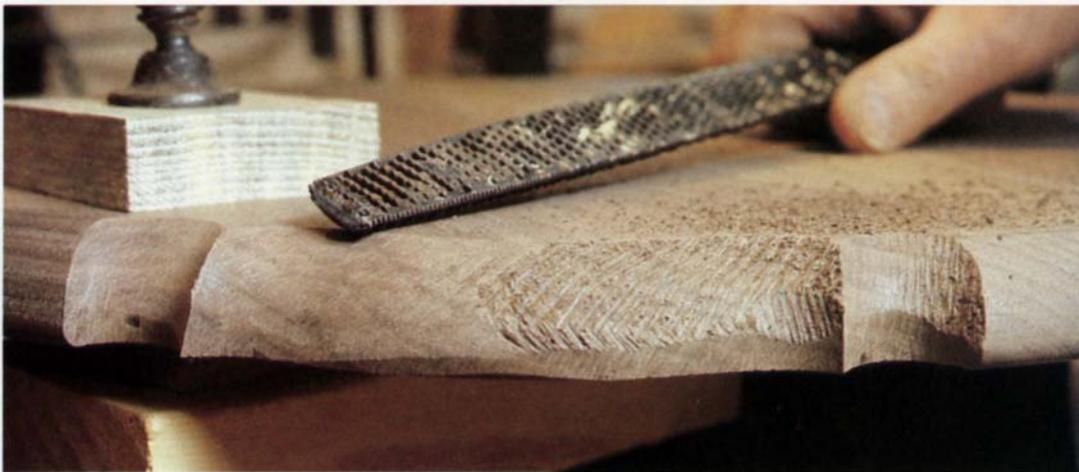
**16.** Here's the idea on the back. Rough out with a coarse rasp, then finish up with ever-finer rasps and files until the wood shimmers. You'll probably find that the back has warped as a result of the dish on the other side. This is no problem, because the surface ought to be planed flat anyway, when the glue block is removed.
