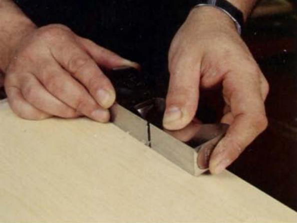
5. Clean up tearout at the field's shoulder with a shoulder plane laid on its side. The shoulder plane can also be used to trim the bevel, but a block plane works better.
