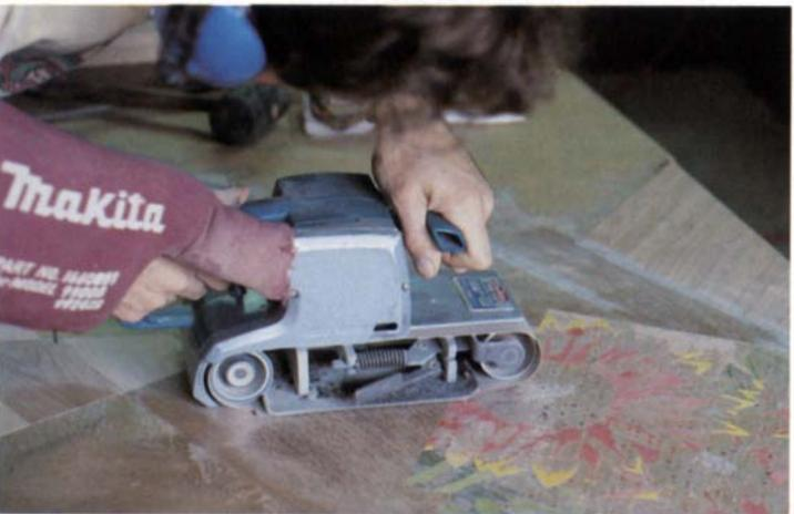
*The completed marquetry is glued to the panel, then sanded and leveled with a belt sander and a worn 120-grit belt.*
