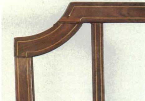
*This delicate chair is a visual treat, but the narrow, short grain in its curved elements is prone to breakage.*
