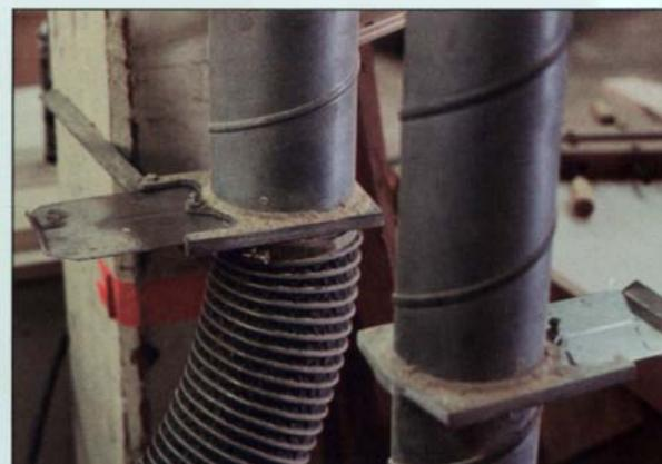
*Above left, Verner Peer of Summit, N.J., turned a handful of plugs on his lathe to act as blast gates. Commercial blast gates, right, shut off duct leading to an industrial Torit dust collector at Coastal Woodworking of Bridgeport, Conn.*
