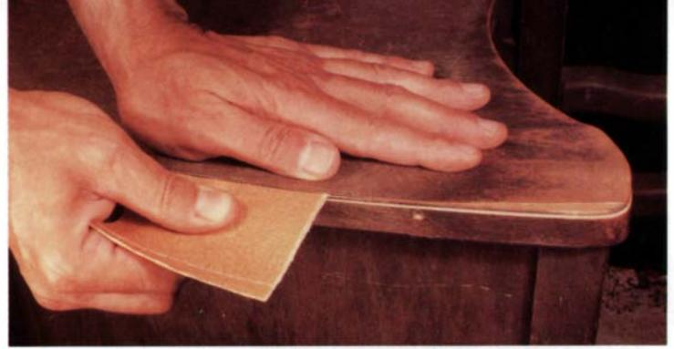
*To remove glue from under loose veneer, fold sandpaper in half and slide it back and forth while pressing lightly on the top surface of the veneer.*
