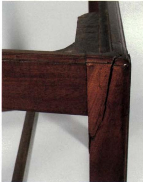
*Grain running off the end of this chair post indicates a weak area that almost certainly will be pulled apart by stress on the mortise and tenon joining the rail to the post.*
