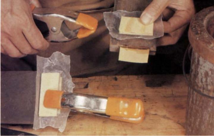
*A loose tenon can be built out to fit its mortise by gluing on a piece of veneer or a strip of wood. Clamp the piece down with a wooden block protected from glue squeeze-out by wax paper.*
