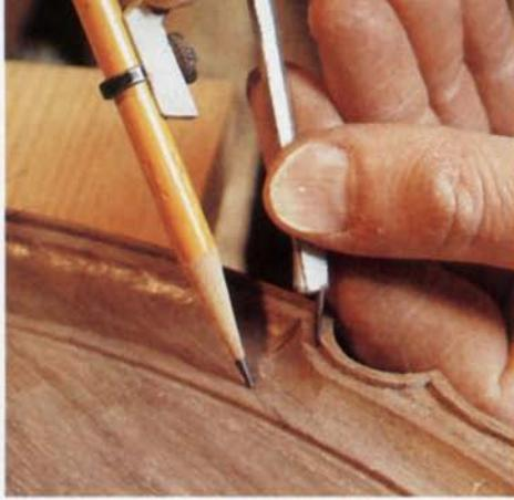
**12.** The next four photos show a critical part of the carving, extending the flat top up to the cove. Marking out is done with a compass, then stop cuts are made with chisels and gouges. Be careful not to make your stop cuts too deep, or they will mar the look of the top. The trick is to work the flat down gradually.
