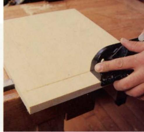
3. A rabbet plane cuts the perimeter of the raised field. The scrap clamped to the edge of the piece prevents tearout when planing across the grain.
