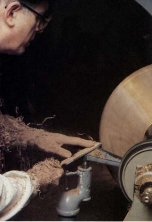
**1.** With my lathe turning at its slowest speed, about 700 RPM, I flatten the back and round the outside edge with a gouge, then clean the surface with a skew used as a scraper. This produces dust from the endgrain areas, but pretty good shavings from the long grain.
