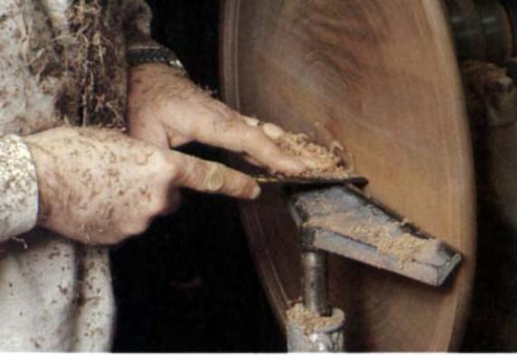
**6.** With the top cut to final depth, tool marks can be removed by scraping. I made this tool from a power-hacksaw blade—there's a clear view of it in photo 15. It has a slightly convex edge, and I use it with the burr left by the grinding wheel.
