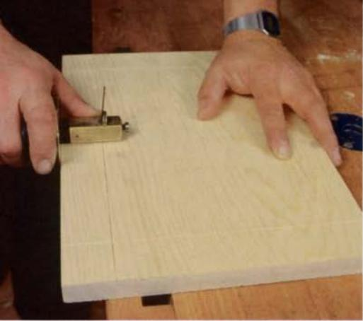
1. The face of the panel is marked with a cutting gauge, both with and across the grain. The rectangle left by the marks is the area to be fielded.
