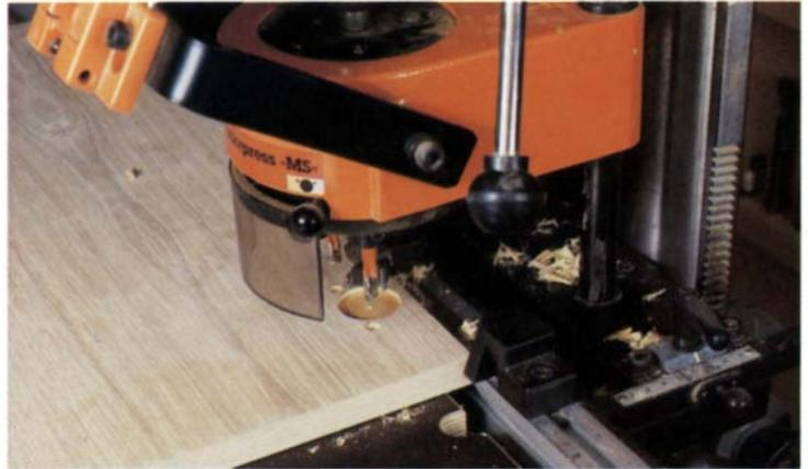
*A low-cost drill-press attachment does double duty by boring three screw holes simultaneously and then pressing the hinge in place on the cabinet door.*
