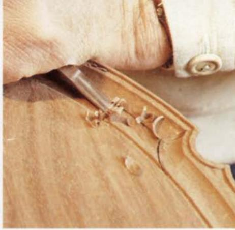
**13.** The first cuts, made with a #2 gouge, can be fairly bold, similar to the way in which the roughing cuts were made when carving the cove. But be somewhat cautious. There's a real danger of going too deep and making a depression between the flat top and the cove. This will absolutely ruin the look of the table.
