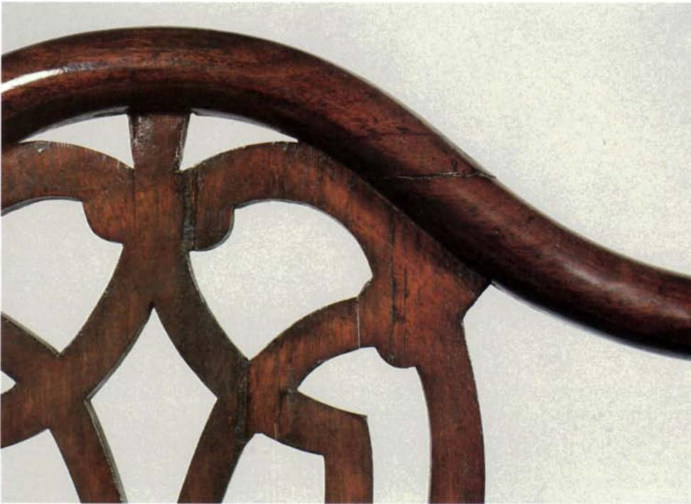
*The long grain of the crest rail restrains the normal cross-grain movement of the pierced back, increasing the chances of breakage in thin, decorative elements.*
