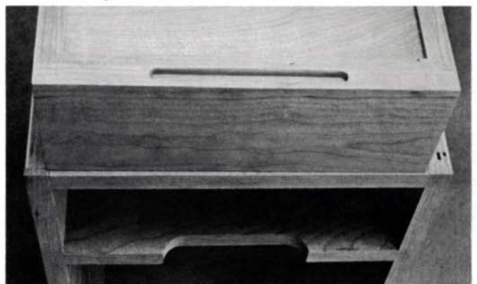
A finger pull that Frid routed in the drawing-table drawer front would have exposed the groove into which the plywood bottom is normally let—a problem Frid solved by gluing a slip to the front, as well as to the sides. The carcass rail, visible at the bottom of the photo, is relieved to give access to the pull.
