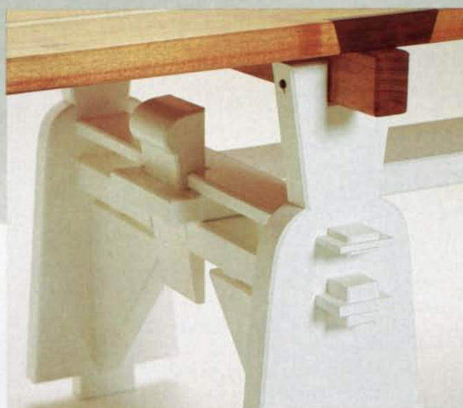
Acacia trestle assemblies, painted white, support a knotty acacia top. The long, wedged stretcher is shouldered top and bottom for a snug fit between the parallel crosspieces, whose slotted ends receive glued-in blocks that lock the trestles together.
