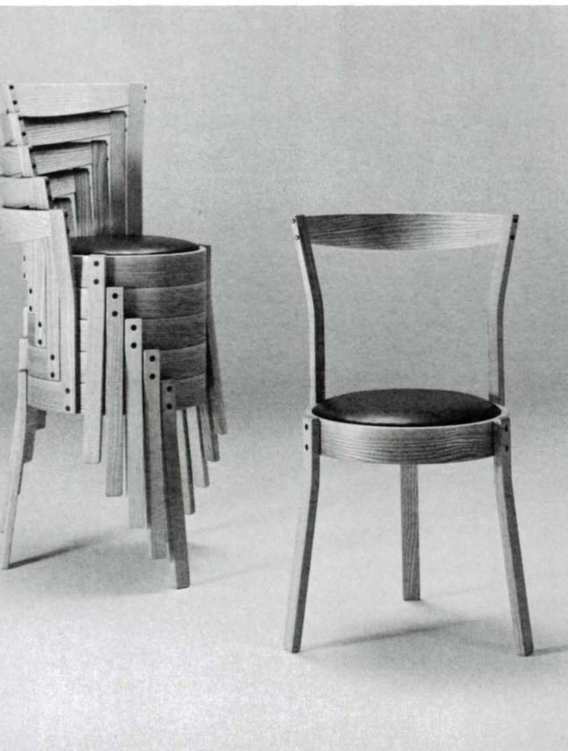
In these knockdown spiral-stacking chairs, every piece was laminated and bent, then joined together with metal fasteners.
