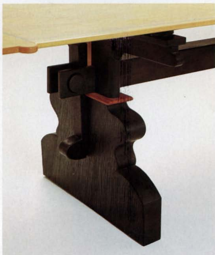
A brisk scrub with coarse steel wool cleans up the chainsawn surfaces of this walnut pedestal, above. Then Bennett dyes the wood black, applies paste wax, and burnishes with a hardwood stick. Right: Wedge bears against cam that's pinned into bamboo stretcher.
