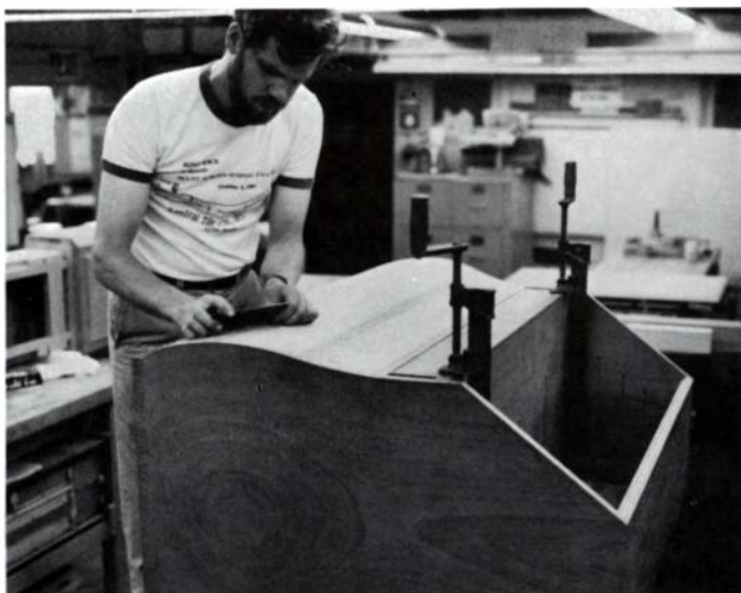
Jerry de Rham, a student at North Bennet Street School, scrapes his desk front smooth. Note the alternate traditional design—the front is not serpentine, but matches the curve of the sides.
