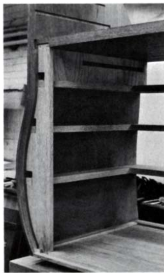
Notched vertical members support drawer runners at back.
