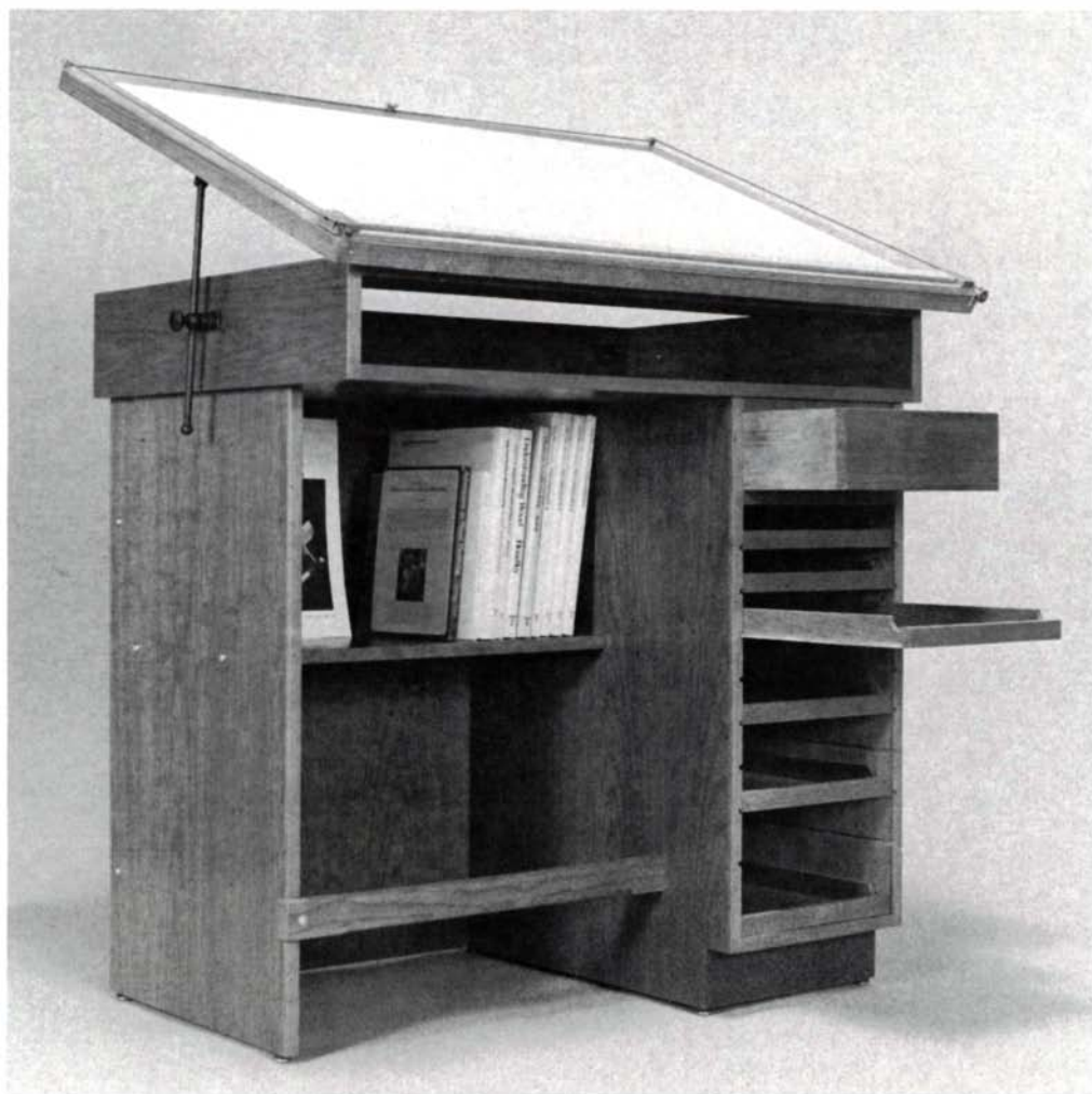
The small, conventional drawer and five shallow trays in Frid's compact, knockdown drawing table provide plenty of storage, and illustrate the basic drawer-making techniques that you can apply to any kind of furniture.
