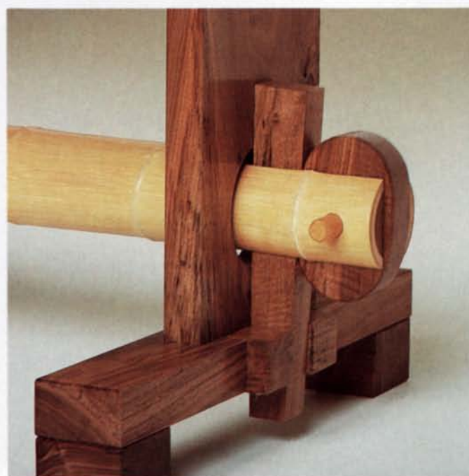
A brisk scrub with coarse steel wool cleans up the chainsawn surfaces of this walnut pedestal, above. Then Bennett dyes the wood black, applies paste wax, and burnishes with a hardwood stick. Right: Wedge bears against cam that's pinned into bamboo stretcher.
