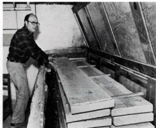
Klimesh loads his kiln with green, 2-in. pine boards.
